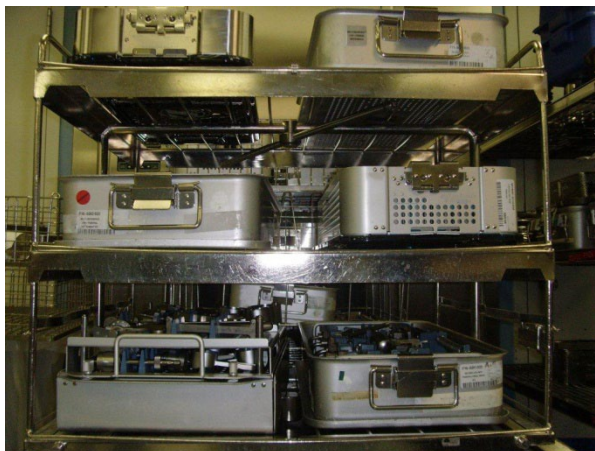
Figure 17 – Overloading/Incorrect Loading of Instrument Trays and Sets
