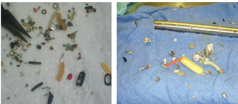
Figure 15 – Debris Found Inside a Single Spray Arm
