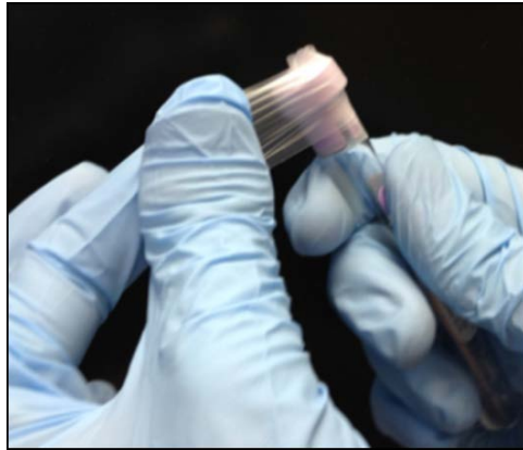
Each specimen is sealed with paraffin film.
